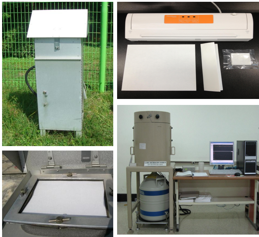
Fig. 2.10 Collection and analysis system for airborne dust sample
