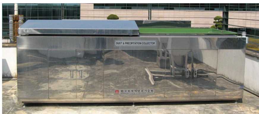
Fig. 2.11 The automatic dust and precipitation collector
