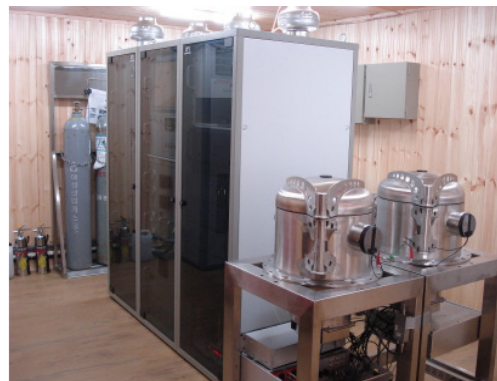
Fig. 5.1 Nuclear event monitoring station(left) and fixed radioactive Xe monitoring system(SAUNA II-IMS, right)
