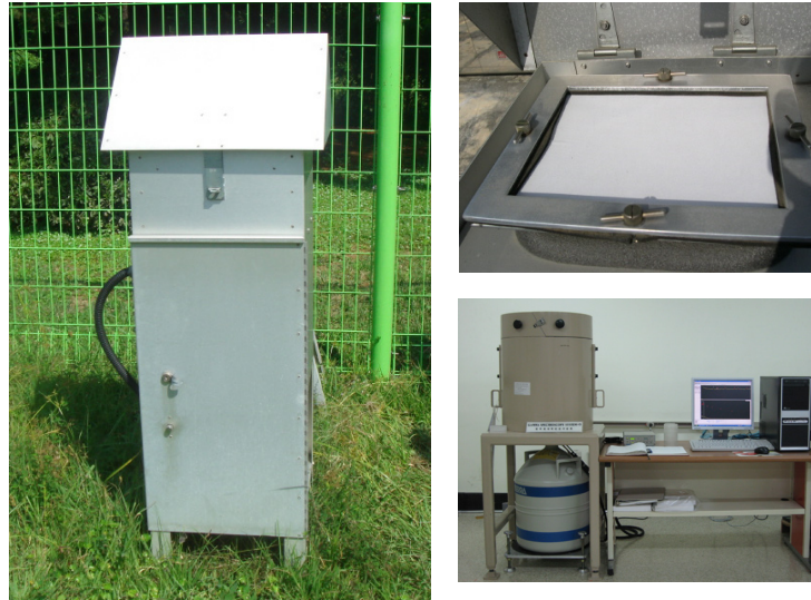
Fig. 2.10 Collection and analysis system for airborne dust sample
