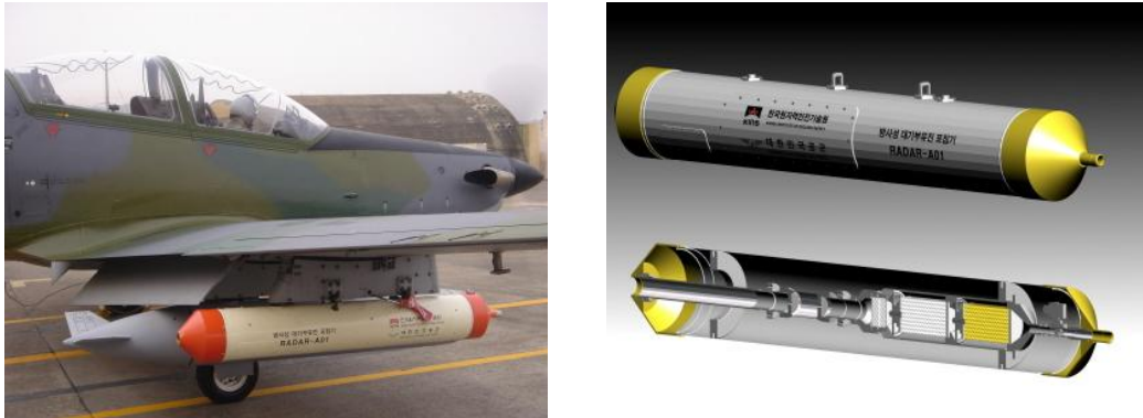
Fig. 5.2 Tactics control fighter(KA-1) and the Radioactive Airborne Dust Archive for Aircraft (RADA-A)
