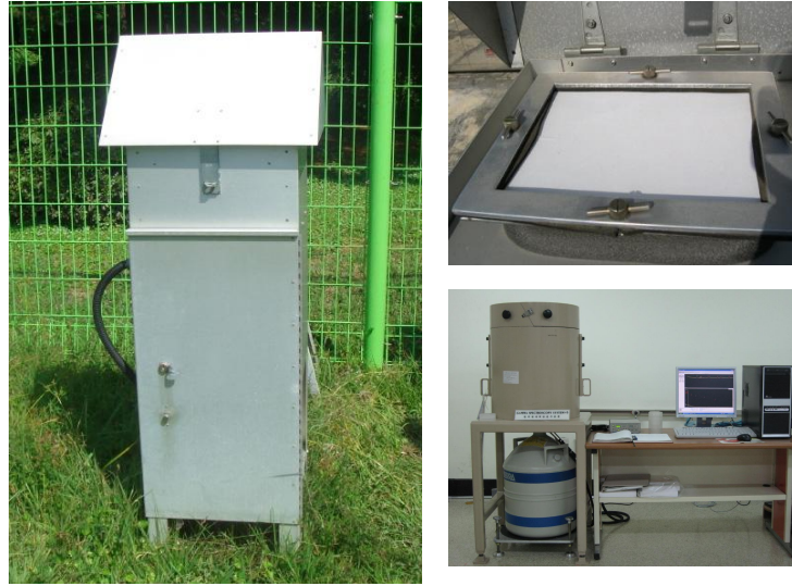
Fig. 2.11 Collection and analysis system for airborne dust sample
