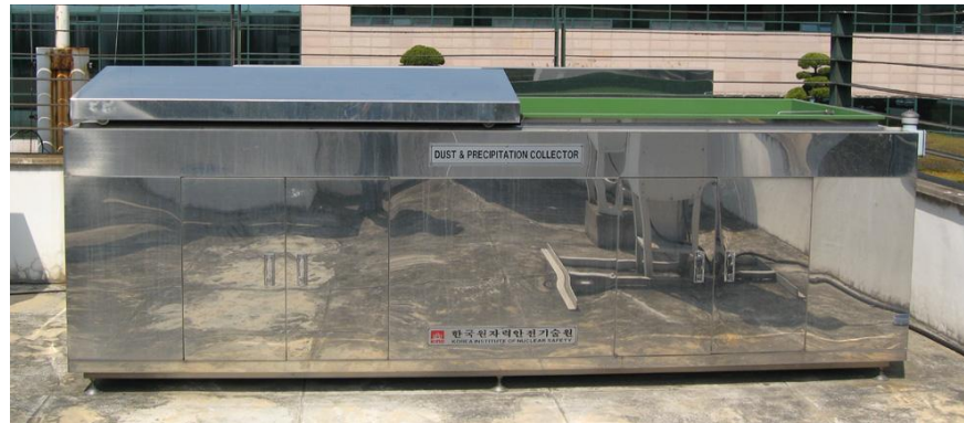
Fig. 2.12 The automatic dust and precipitation collector
